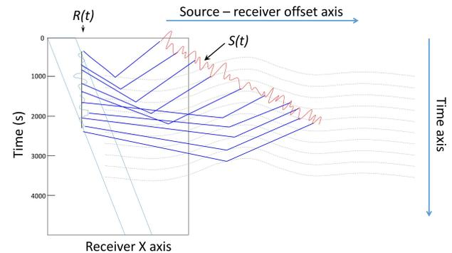
**Figure 2** -  $R(t)$  is a stationary receiver trace as a function of time, and  $S(t)$  are the source signals emitted as a function of time in different offsets relative to the receiver location. The grey dashed lines represent one reflector in the sub-surface, and the blue lines represent some of the ray-paths from the source reflected at the sub-surface reflector and received in the stationary receiver position.
