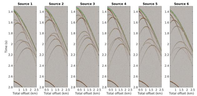
**Figure 5 - Result of deconvolving the source wavefield into six common receiver gathers with earth responses extracted from one stationary receiver location based on the source configuration shown in Figure 4. The spacing between the strings of air-guns was 200m.**
