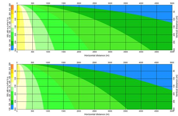
**Figure 8 - Sound exposure levels (in dB re 1 µPa²s) as a function of distance from the source. Horizontal axis is meters from the geometrical center of the array directly aft from the vessel, while the vertical axis is depth from the sea surface in meters. The integration time is set to 10 seconds starting from the first arrival at each location. Conventional 4130 cubic-inch array (top) is compared with triggering individual air-guns in a near-continuous fashion on the bottom.**
