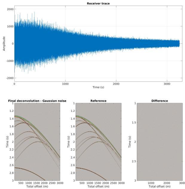
**Figure 3 - Top:** Simulated receiver trace in a stationary position containing more than 3000 seconds of signals received continuously. **Bottom:** Results from the iterative source deconvolution process shown to the left. The image in the middle shows the desired output, and the image to the right shows the difference between the deconvolution result and the desired result.
