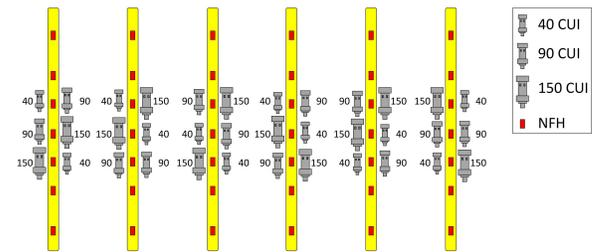
**Figure 4 - Six strings with 40, 90 and 150 cubic-inch air-guns on each. The configuration of the three volumes is different on each sub-array to provide additional encoding of the wavefield emitted from each string.**
