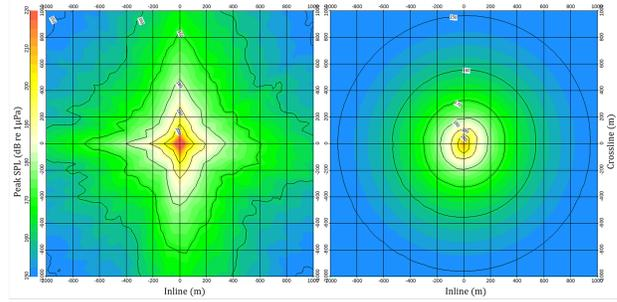
**Figure 7 - Peak sound pressure levels (in dB re 1 µPa) as a function of inline and cross-line distances in meters from the geometrical center of the source at a depth of 10 m (4 m below the source depth) for a conventional 4130 cubic-inch array (left) and when triggering individual air-guns in a near-continuous fashion (right).**
